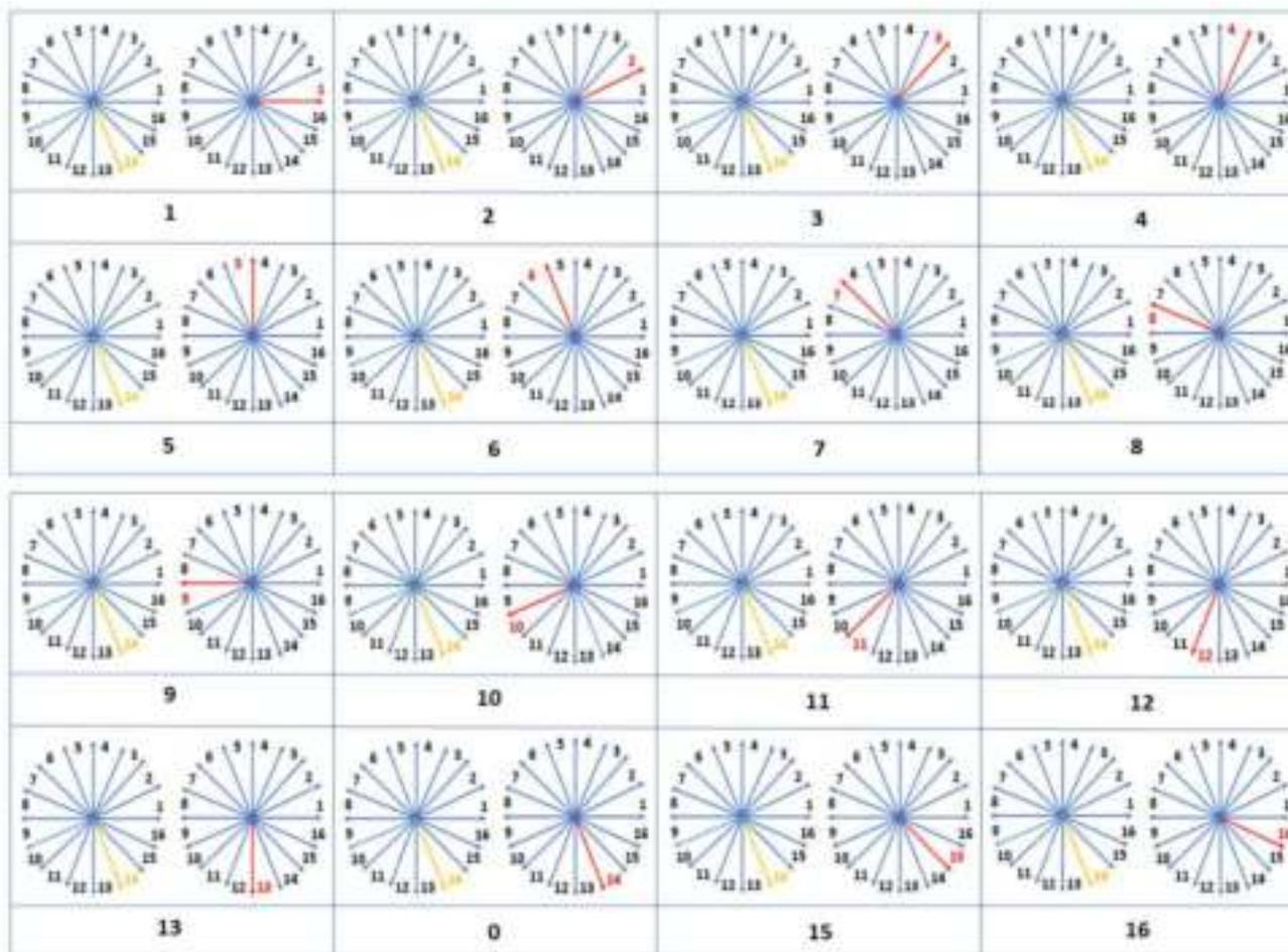
**FIGURE 5.** Calculation of texture orientation-based pattern values for the center pixel direction ‘14’ based on the direction of surrounding neighbors. The yellow line represents the center pixel direction, while the red line represents the direction of surrounding neighbors.
