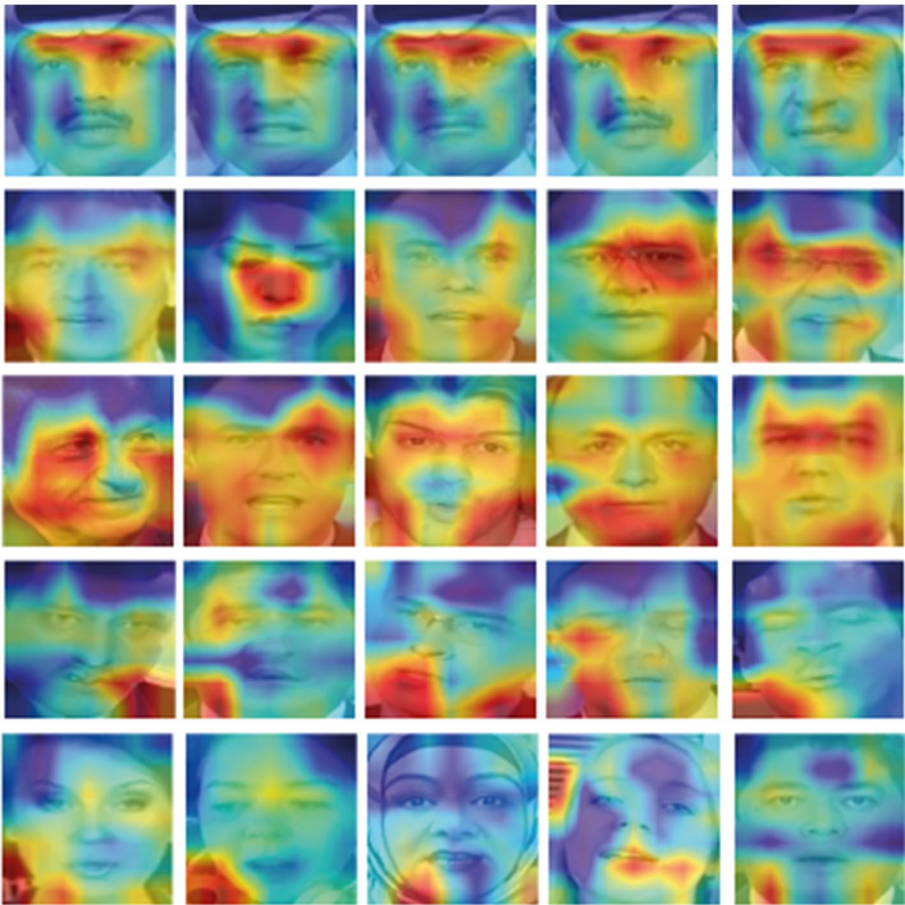
Fig. 9 Each column has different samples of FS, DF, F2F, NT, and SH subsets of FF++ datasets. 1st row represents heat maps without post-processing attack, 2nd row represents noise attack heat maps, 3rd row represents blur attack heat maps, 4th row represents pixel dropout attack heat maps, and 5th row represents elastic deformed attack heat maps
