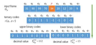
Fig. 2. Acoustic Local Ternary Pattern (acoustic-LTP) Computation.
