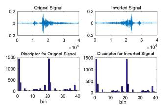
Fig. 6. Descriptors for original and inverted signals.
